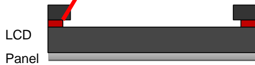
Frame bonding - Bonding frame to Display module
